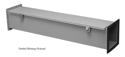
Construction: C & I Enclosures Type 4X Stainless Steel Feed-Through Wireway is fabricated in accordance with U.L. specifications from code gauge material. An oil resistant gasket is attached to the cover to prevent dust from entering the wireway. The cover is attached to the body with butt hinges on one side and external screw clamps on the other. All seams are continuously welded and ground smooth.
